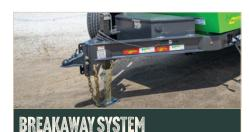
The safety breakaway system with cable ensures your dump trailer stops safely if it disconnects from the towing vehicle, preventing accidents and keeping your load secure.
