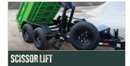
In dump trailers, scissor lifts provide powerful, stable lifting for heavy loads, ensuring smooth and efficient dumping operations. Their design allows for balanced weight distribution, enhancing safety and reliability during use.
