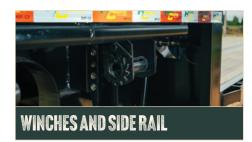
Our Beavertails offer evenly spaced stake pockets and movable winches (12) and feature 3/8" X 2-1/2" steel rub rails and 6" steel channels.
